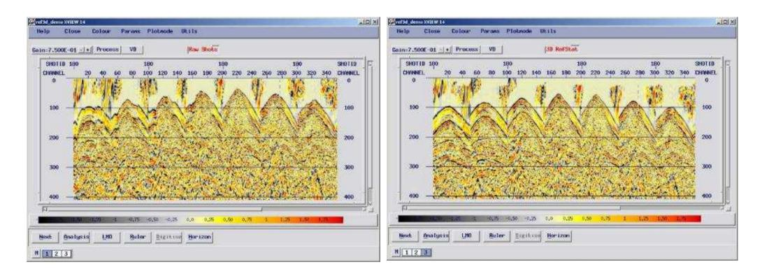
The RefStat approach is equally effective on 3D data or where the issue is low near surface velocity anomalies of varying thickness
