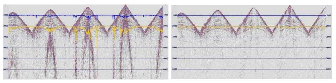
Interactive analysis tools and the ability to spatially vary workflows allows users to rapidly optimise the quality of pre-stack land or marine seismic data.
