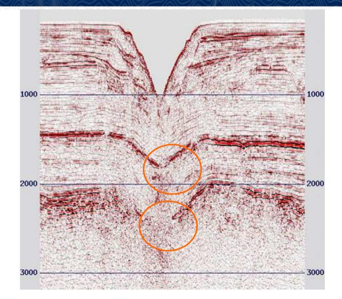
GLOBE Claritas<sup>™</sup> seismic processing software Original post stack migration
