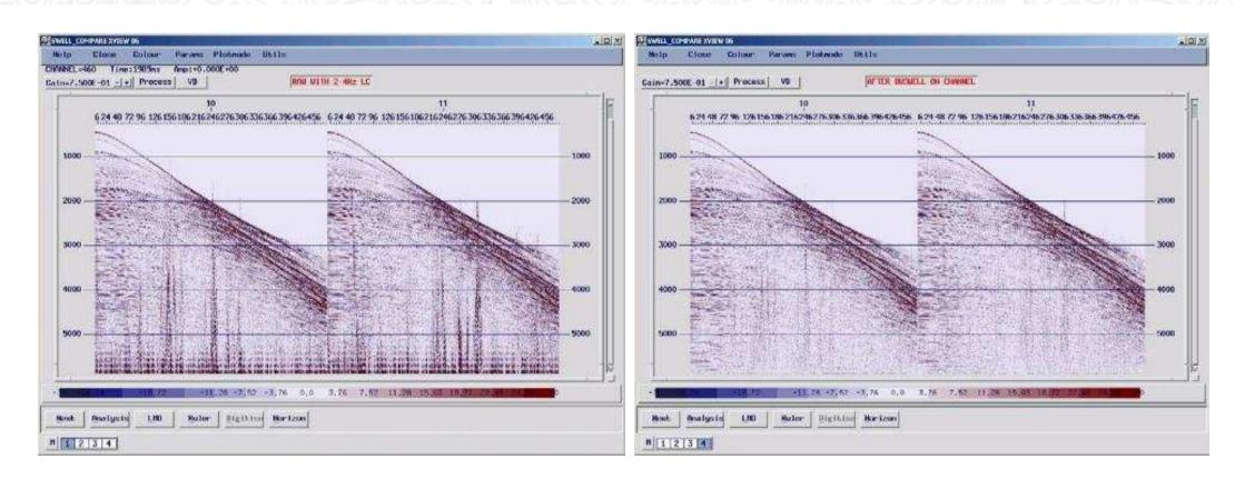
DUSWELL removes swell-noise trains from the data without compromising the overall frequency content. Like most modules, it can be run in parallel on any number of cores/CPUs.
