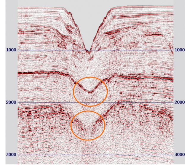
GLOBEClaritas<sup>™</sup> seismic processing software Pre-stack Time Migration using HDVA velocities
