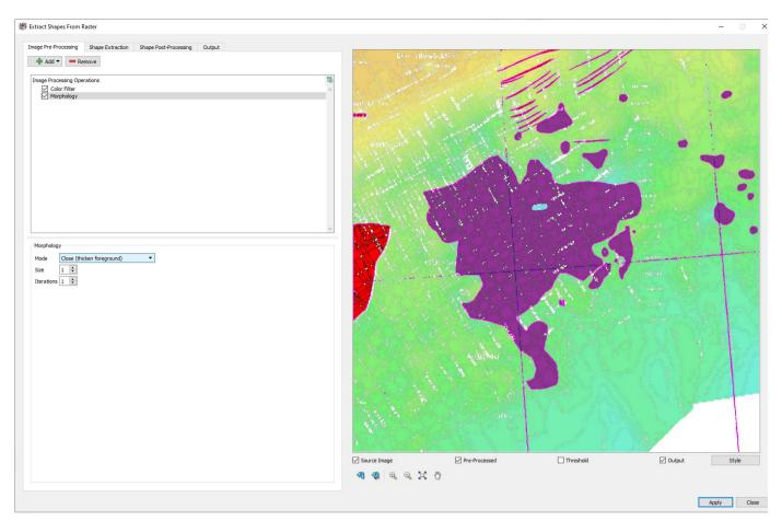
Image processing is applied to remove the seismic lines, faults on the map image (shown above). Then the users highlights the polygons from the image – shown below in the threshold bitmap view (black and white). These resulting polygons are extracted and can be saved to a variety of file formats supported by our spatial data outputs, eg shapefiles, geodatabases, 3<sup>rd</sup> party data sources, etc.
